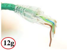
Place Grn pair and bend back @  $90^{\circ}$  like lower pairs
