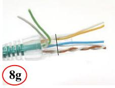
Untwist lower three pairs back to ends of side walls
