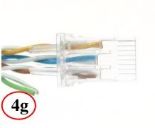
First insert Org, Blu, Brn pairs into lower row of load bar, then insert Grn into upper row
