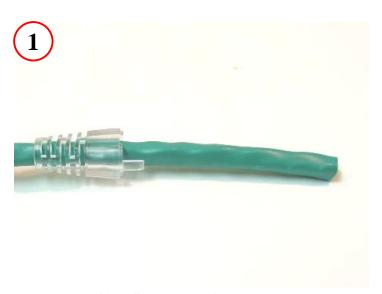
Slide Strain Relief onto cable
