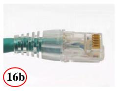
Snap housing and load bar assembly together
