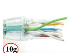
Check Grn pair for alignment Add ½ twist if necessary
