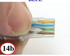
Trim wire ends flush with end of load bar
