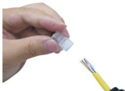
**Step 4:** Put the RJ45 connector in place with cable crimper.
