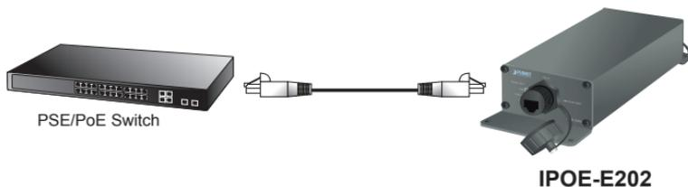
**Step 2:** The PSE delivers both Ethernet Data and PoE power over UTP cable to the IPOE-E202 and the “**PoE IN**” LED will be lit steadily.
