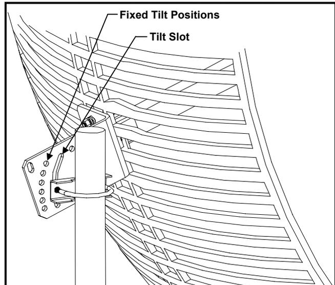
To mount antenna assembly in a tilted position, attach (1) U-Bolt assembly to either the fixed tilt positions or to the tilt slot (as shown) on the “L” Bracket.
