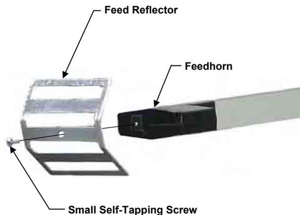
**Install the Feed Reflector to the front of the Feedhorn using the small self-tapping screw.**
