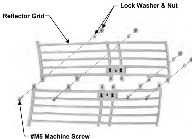
**Assemble the halves of the Reflector Grid using (4) #M5 machine screws with lock washers, flat washers and nuts as shown.**
