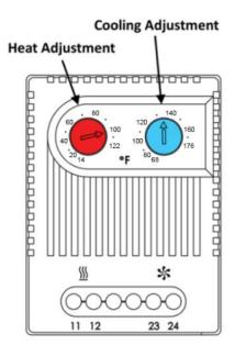
The cooling thermostat features a Normally Open (NO) circuit. When the temperature rises to the temperature set on the cooling adjustment dial the circuit closes which turns on the cooling fans. When the temperature falls below the temperature set on the cooling adjustment dial the circuit opens which turns off the cooling fans.
