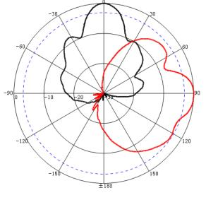
Freq:4900MHz Date:2013-11-20 Elevation:H-plane Polar-Across:Main Polarization:Vertical Max:-18.64dB HPBW(3dB):22.60° FBR:27.59dB
