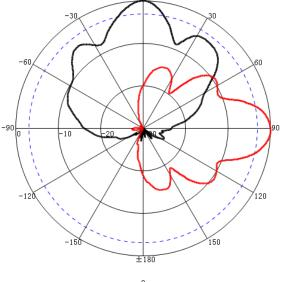
Freq:4900MHz Date:2013-11-20 Elevation:H-plane Polar-Across:Main Polarization:V-plane Max:-16.33dB HPBW(3dB):22.77\* FBR:27.01dB
