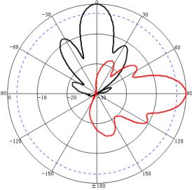
Freq:5400MHz Date:2013-11-20 Elevation:H-plane Polar-Across:Main Polarization:Vertical Max:-18.61 dB HPBW(3dB):18.99\* FBR:31.50dB
