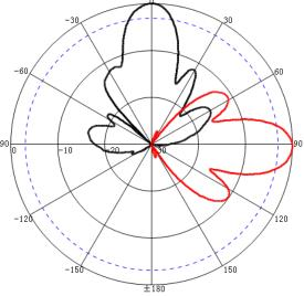
Freq:5400MHz Date:2013-11-20 Elevation:H-plane Polar-Across:Main Polarization:V-plane Max:-18.24dB HPBW(3dB):19.56° FBR:32.24dB
