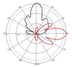
Freq:5850MHz Date:2013-11-20 Elevation:H-plane Polar-Across:Main Polarization:V-plane Max:-20.68dB HPBW(3dB):19.40° FBR:32.88dB
