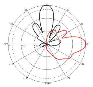
Freq:5850MHz Date:2013-11-20 Elevation:H-plane Polar-Across:Main Polarization:Vertical Max:-21.89dB H-PBW(3dB):19.29° FBR:31.32dB
