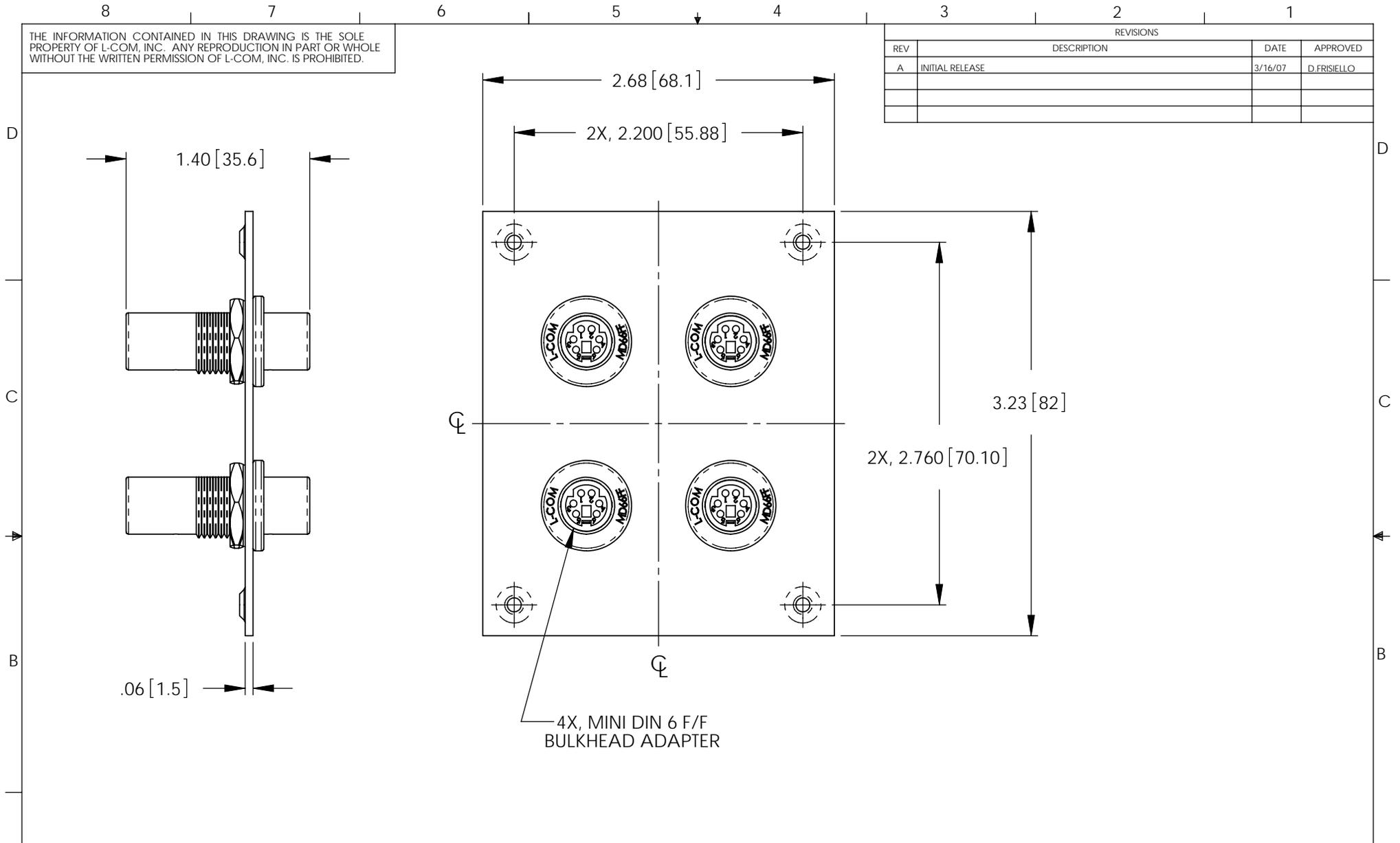
4X, MINI DIN 6 F/F BULKHEAD ADAPTER
