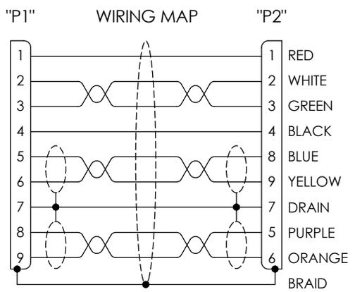
(2) TWISTED PAIR, 26AWG WITH ALUM/POLY FOIL SHIELD AND DRAIN WIRE,
