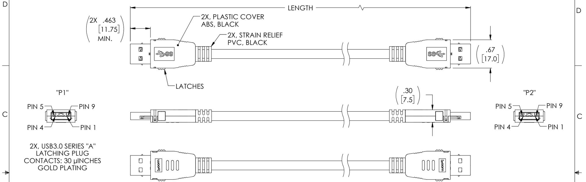
2X, USB3.0 SERIES "A" LATCHING PLUG CONTACTS: 30 μINCHES GOLD PLATING
