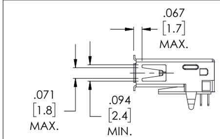
RECOMMENDED SIDE NOTCH SIZE FOR MATING A FEMALE CONNECTOR
