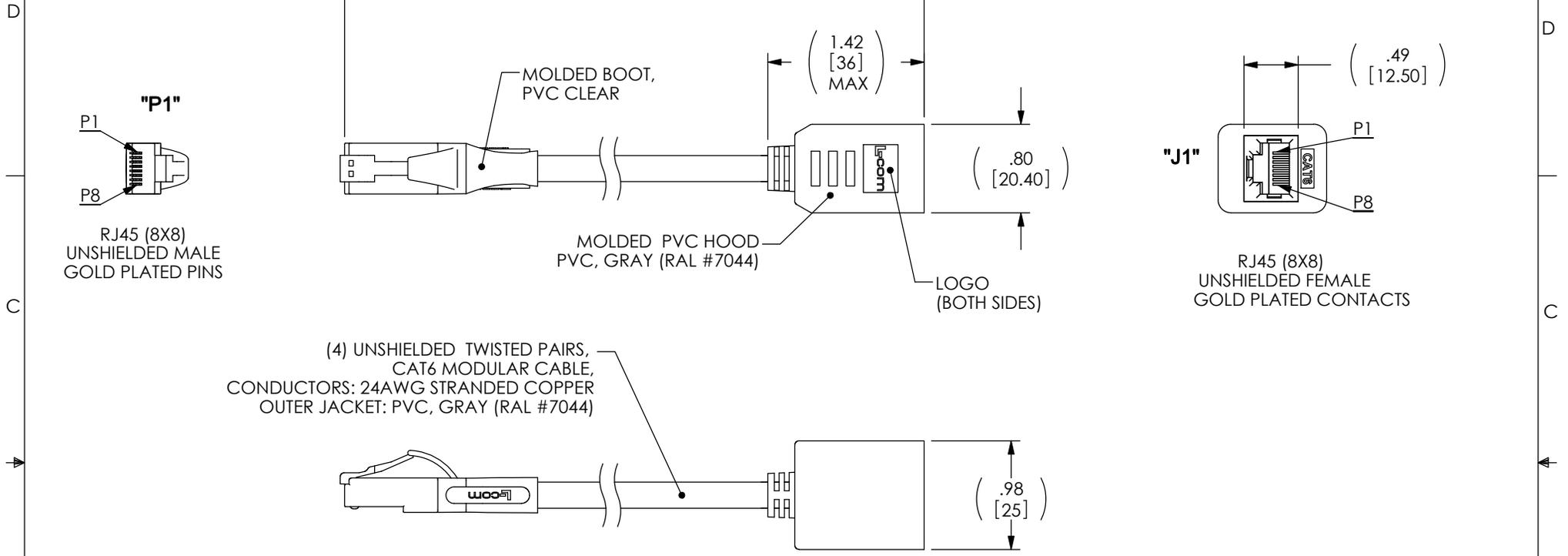
(4) UNSHIELDED TWISTED PAIRS, CAT6 MODULAR CABLE, CONDUCTORS: 24AWG STRANDED COPPER OUTER JACKET: PVC, GRAY (RAL #7044)
