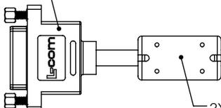
2X ENCAPSULATED FERRITE BEAD, PVC, GRAY (PANTONE 424C)
