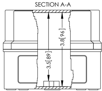
THRU HOLES FOR MOUNTING ENCLOSURE USING #6 SCREWS (4X)
