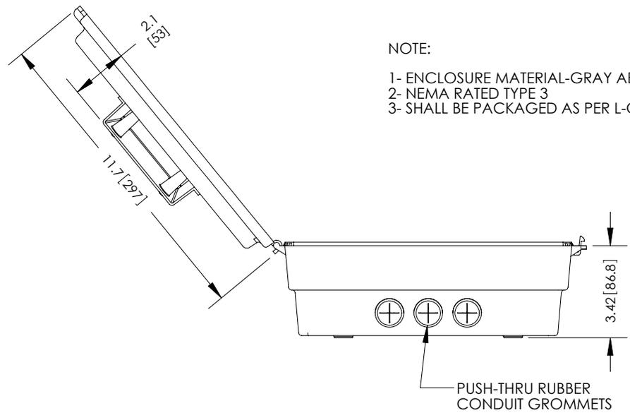
PUSH-THRU RUBBER CONDUIT GROMMETS
