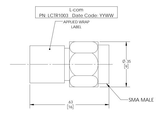
UNLESS OTHERWISE SPECIFIED LEADING DIMENSIONS ARE INCHES DIMENSIONS IN [] ARE MILLIMETERS TOLERANCES: .X=± .2 [5.08] FRACTIONS .XX=± .01 [.25] ± 1/32 .XXX=± .005[.13] ANGLES ± 1° ALL DIMENSIONS SHOWN ARE FOR REFERENCE ONLY.
