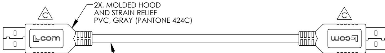
ONE 28AWG STRANDED TINNED COPPER TWISTED PAIR
