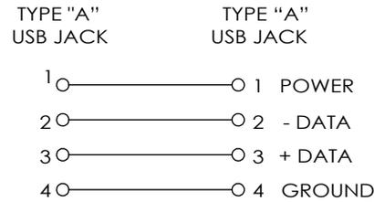
CONNECTOR SHELL ————— CONNECTOR SHELL
