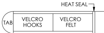
STRAP IS LOOPED THROUGH SLOT ON BRACKET OF THIS TELCO CONNECTOR AND HEAT SEALED
