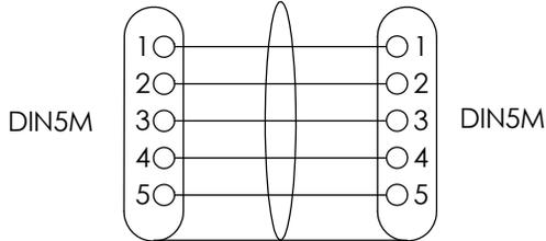
CABLE SHIELD DRAIN WIRE IS CONNECTED TO BOTH DIN SHELLS
