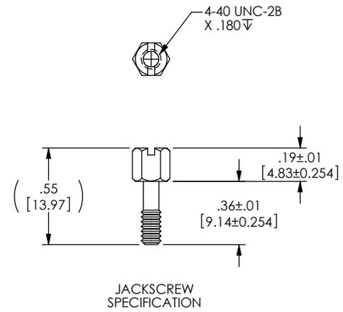
**NOTE: DIFFERENT STANDOFFS AND JACK SCREWS ARE REQUIRED FOR PANEL MOUNTING. SEE WWW.L-COM.COM OR MASTER CATALOG FOR DETAILS.**
