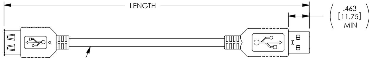
ONE 28AWG STRANDED TINNED COPPER TWISTED PAIR
