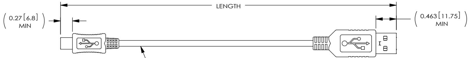
ONE 28AWG STRANDED TINNED COPPER TWISTED PAIR
