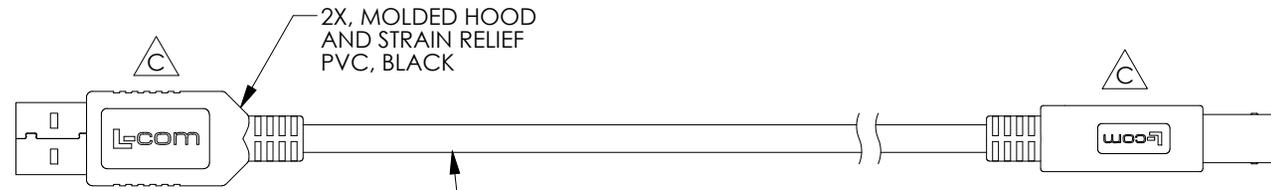
ONE 28AWG STRANDED (19X40) TINNED COPPER TWISTED PAIR
